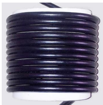
Figure 2: The minimum 160m and higher ugly balun.
