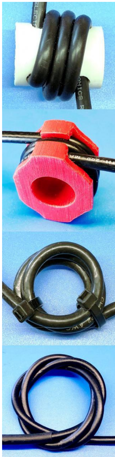
Figure 1: a: neatly wound on a form: b: a handy quick form, c: scramble wound with zip ties, d: scramble wound as a torus knot
