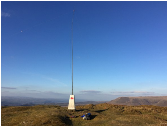
Trig point as antenna mast support
