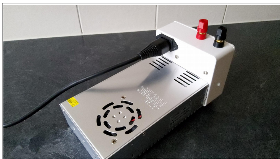
Power input socket fitted Power lead with fused plug
