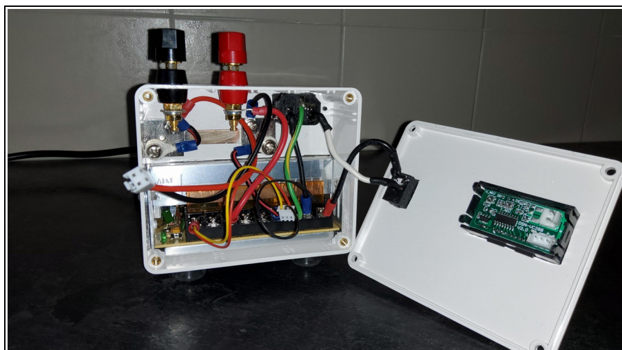
You can see the 50Amp meter shunt in the bottom of the box. The sampling leads go to a plug that fits on the 2 pins on the meter board. The yellow, red and black wires power the meter, with the yellow being the voltage measurement wire. In this configuration the black is not required.
