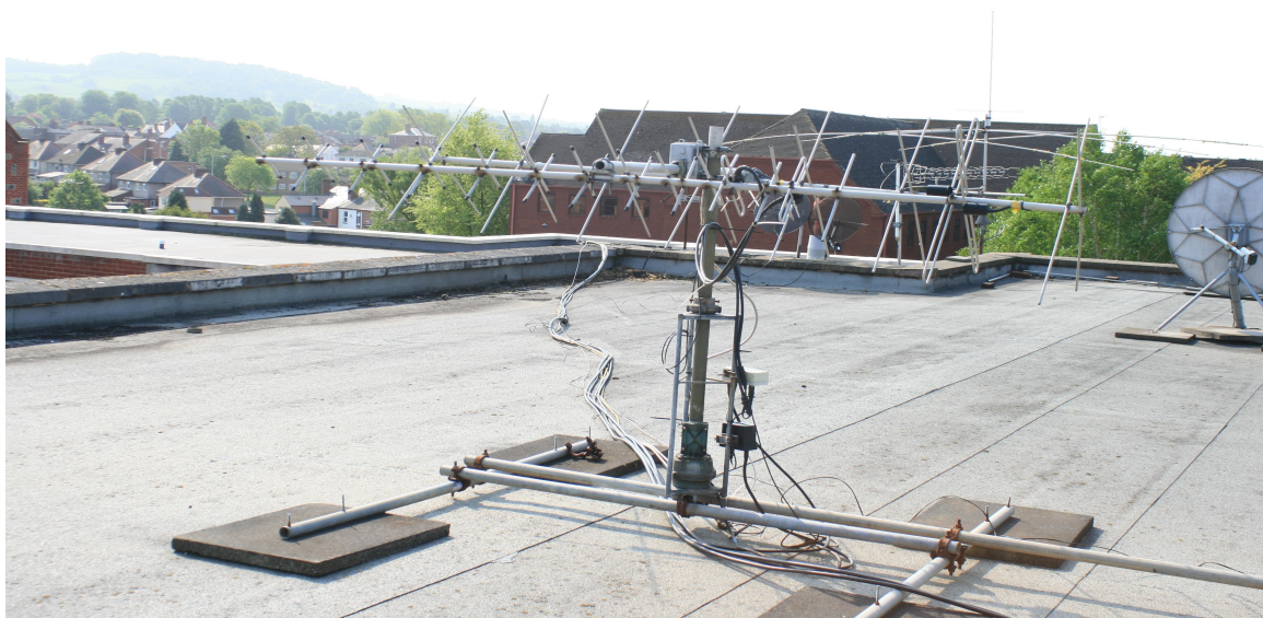
Bayed 2 metre with crossed yagi with azimuth control and rotator
