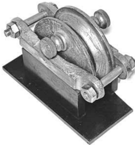
Spark gap from high power transmitter dating from early 1900s.
