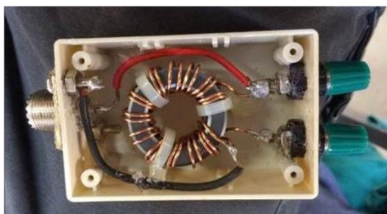
Homebrew 4:1 balun using the Jaycar L15 core with 2 x 10-turn windings
