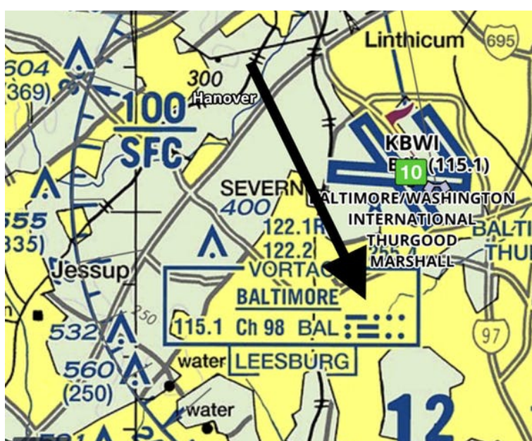
The arrow points at the chart label indicating the Morse code equivalent to the 'BAL' signal for a radio beacon near Baltimore
