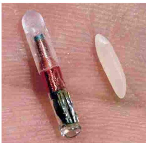
*Illustration 2: Passive RF ID tag compared to a grain of rice. Picture courtesy of Wikipedia*
