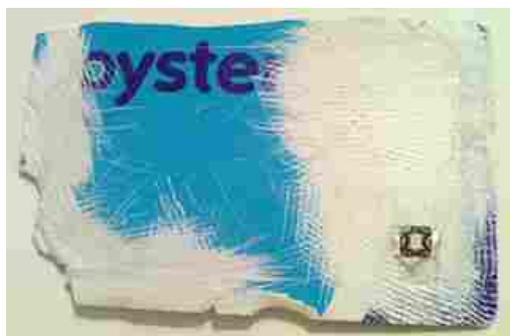
*Illustration 1: An example of a passive RFID tag familiar to travellers on the London Underground. Picture courtesy of tomhannen. Notice the chip and aerial around the edge of the card on this partially destroyed Oyster Card*
